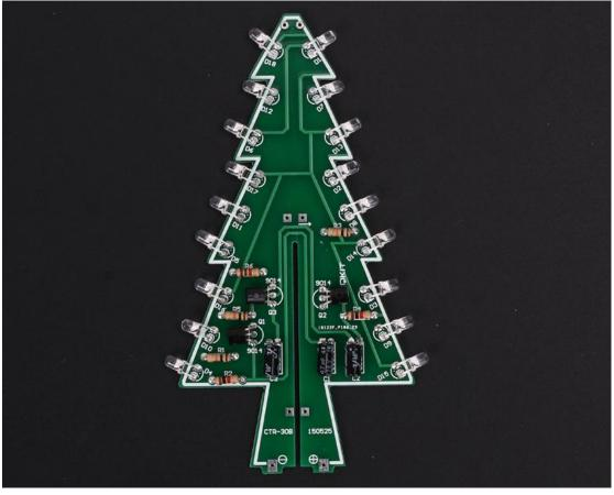
Step 12: Connect 5V to CTR-30A and CTR-30B.Preliminary welding success if LEDs are blinking automatically
