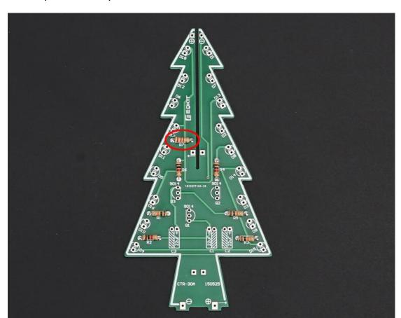
Step 3: Install 1pcs 2.2K Metal Film Resistor on R7
