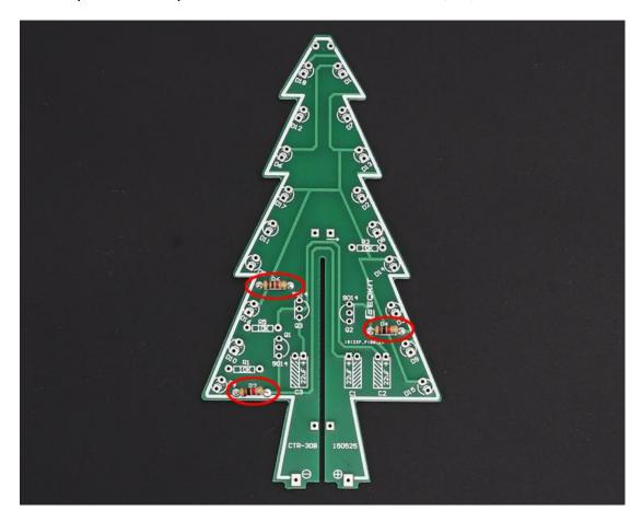
Step 8: Install 3pcs 10K Metal Film Resistor on R1,R3,R5
