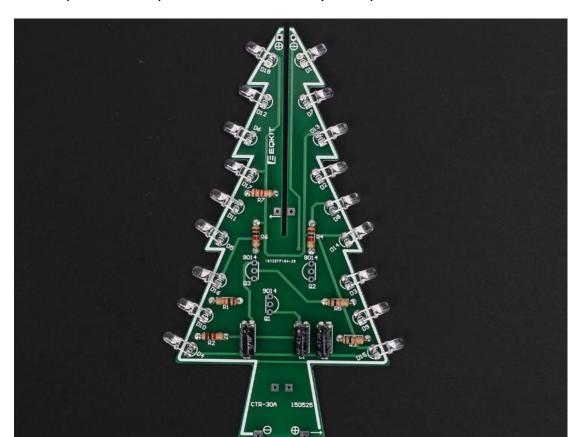
Step 5: Install 3pcs 47uF 16V Electrolytic Capacitor
