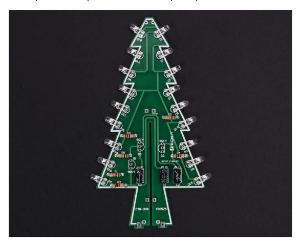
Step 11: Install 3pcs TO-92 S9014 Transistor
