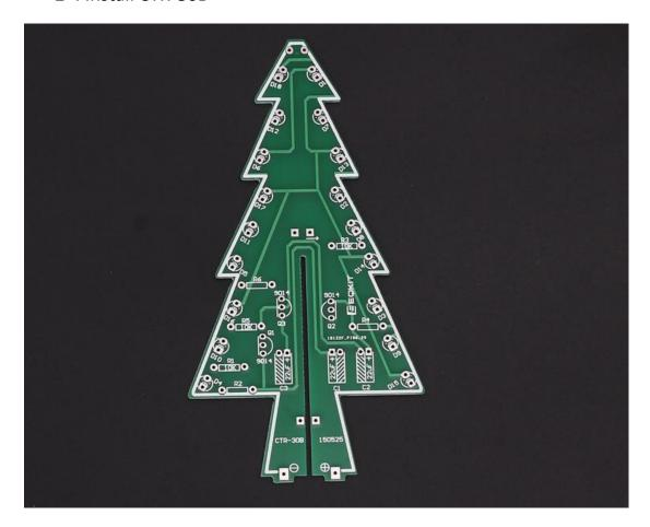
Step 7: Install 3pcs 1K Metal Film Resistor on R2,R4,R6
